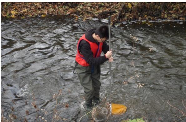
**Figure 2. Kick-Sampling: Hand-net placed on river bed against river flow direction and area around disturbed through kicking.**
